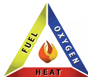
Fire triangle - remove one and you stop the fire
